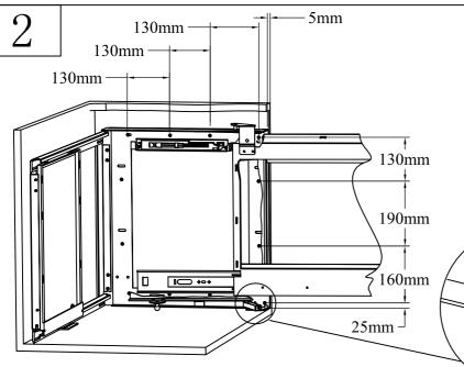
B. Fixing the main inclined frame in frame with screw according to location size as the picture show.
