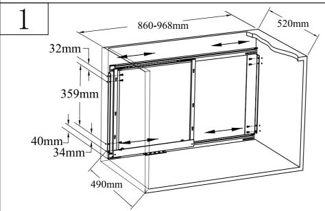
A. Fixing the main slide-out frame in frame with screw accordind to location size as the picture show.
